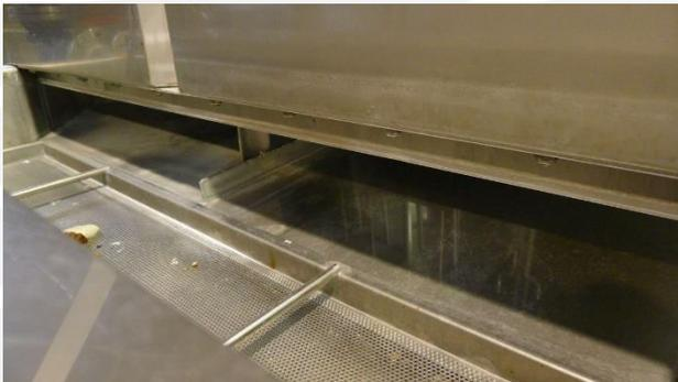
The Cretel rack washer is standard equipped with a static filter which is manually removable for cleaning purposes.
