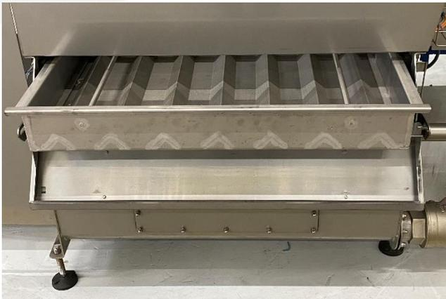
The Cretel cabin washer is standard equipped with a static filter which is manually removable for cleaning purposes. The design is made to create a maximum filtering capacity even in case of intensive soiling.
