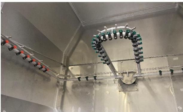
This rotating spraying pattern is motor-actuated and is mounted on the back of the cabin washer. Additionally the loading door is equipped with a built-in fixed or rotating spraying pattern to clean the outside bottom of the items to be washed.
